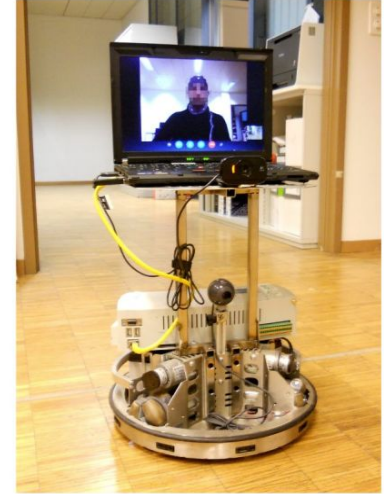
Fig. 1. (left) End-user at a clinic while operating the BCI. (right) The telepresence robot equipped with infrared sensors for obstacle detection and the Skype™ connection on top.
